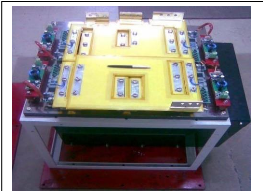
Figure-11(b) Air cooled power module
