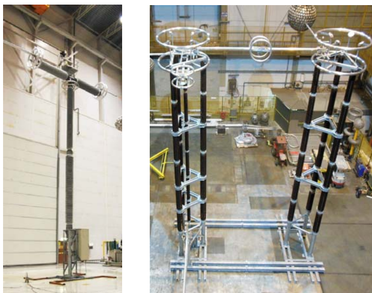
Figure 2 High speed switch 800 kV (left) and disconnector800 kV (right, by courtesy of COELME) during factory testing
