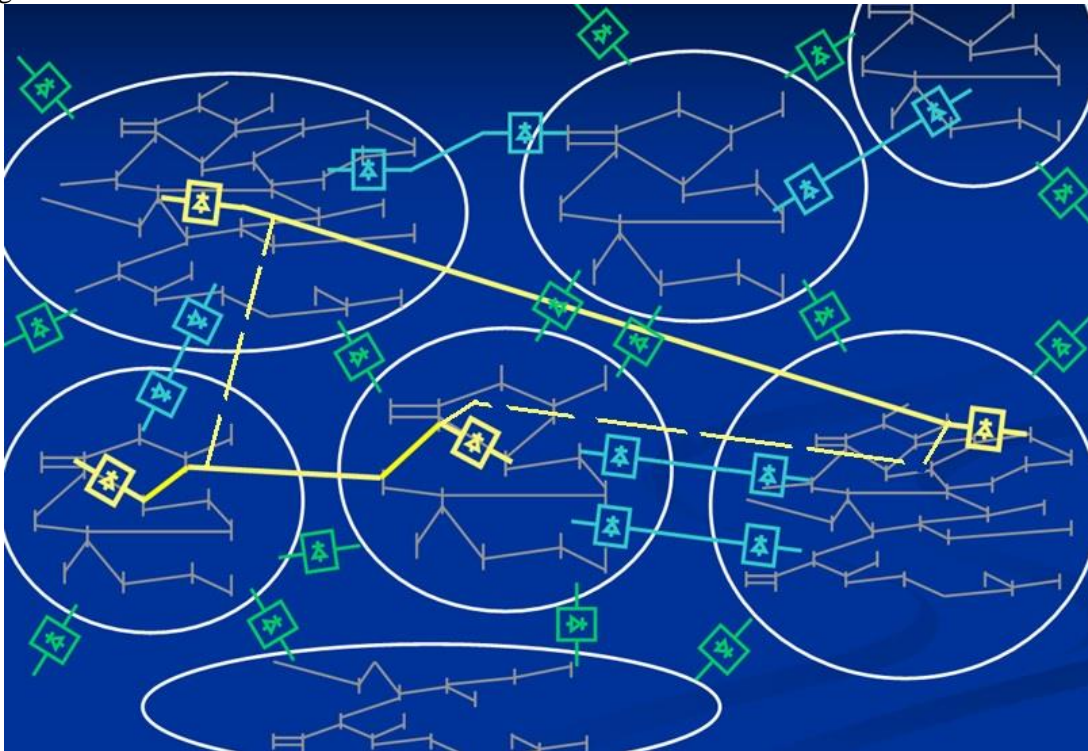
Figure 1. How a segmented AC grid is constructed through back-to-back DC converters (green), AC to DC line conversions or new DC Lines (light blue) , and long distance HVDC lines or DC grid (yellow)
