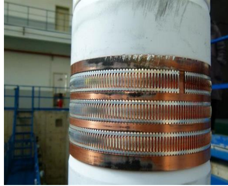
Fig. 12b the marks on the conduct rod
