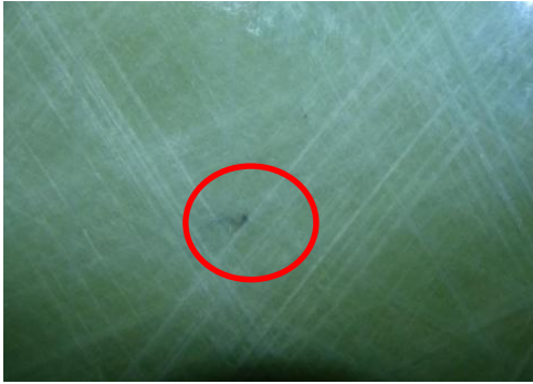
Fig. 12a the pinhole on the Insulator
