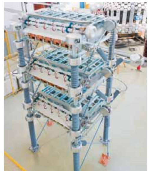
Fig. 21: Dielectric Type Test of HVDC PLUS
