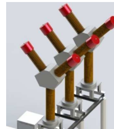
3D model of a high voltage breaker
